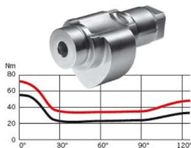
Force profile of an ITS 96 cam action door closer (Size EN 3 – 6, max. closing strength setting)
